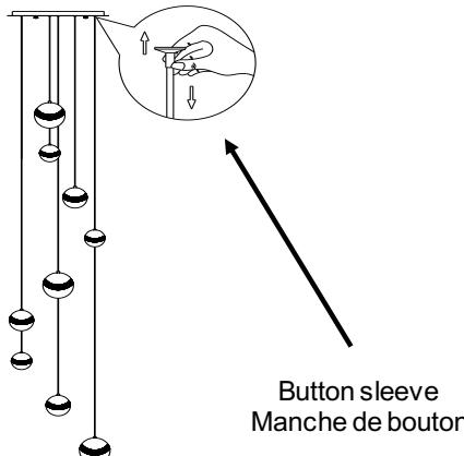
Before installation to ceiling, adjust fixtures to desired length by pushing wire up into canopy, then coiling up excess wire, minor adjustment can be made after installation. To lower or lengthen wire, depress button sleeve located where wire comes out of canopy.
